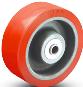
Ergonomic Option 80 Shore A Models Capacity decreases 20% for 80 Shore A durometer models (To order, add 80A to end of wheel number)
