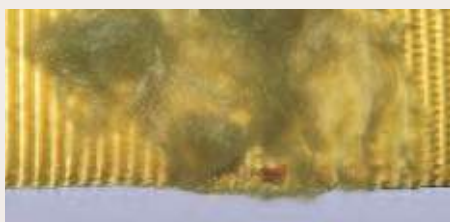
Excessive abrasive wear
